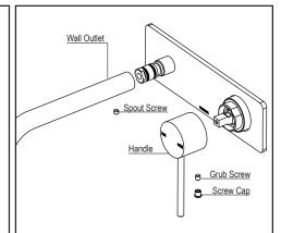
**5** Push Wall Outlet to the spout adaptor and fasten Spout Screws to secure Wall Outlet.
