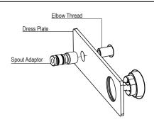
**4** Remove the protective cover from the mixer. Apply Teflon tape to Elbow Thread. Gently, push the dress plate to position. Screw Spout Adaptor to Elbow Thread with a
